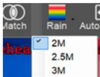
3. Select one of the three default options to the distance between the camera and the testing object/individual. The current image matching will be assigned to the selected distance. Next time the system is launched it will automatically load the last option chosen. .
