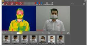
9. Set alarm photo's file location. When temperature screening is in operation, an alarm will be triggered if an individual presents abnormal temperature.
