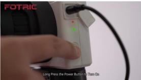
2. Connect the thermal camera to the computer with an USB cable.
